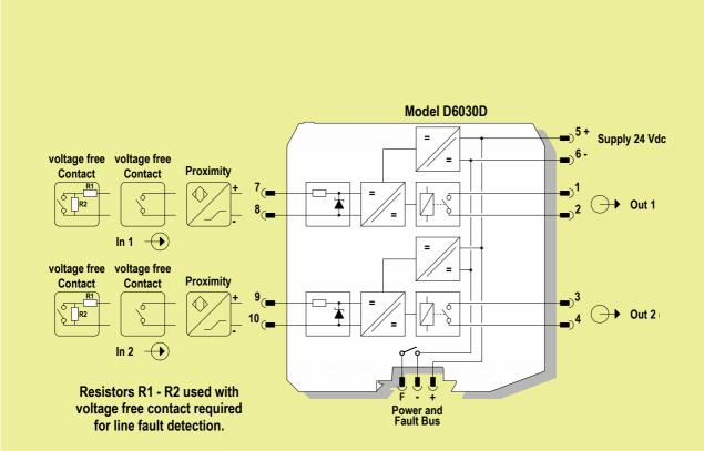
Relay contact shown in de-energized position. Terminals 1-2 and 3-4 open.
